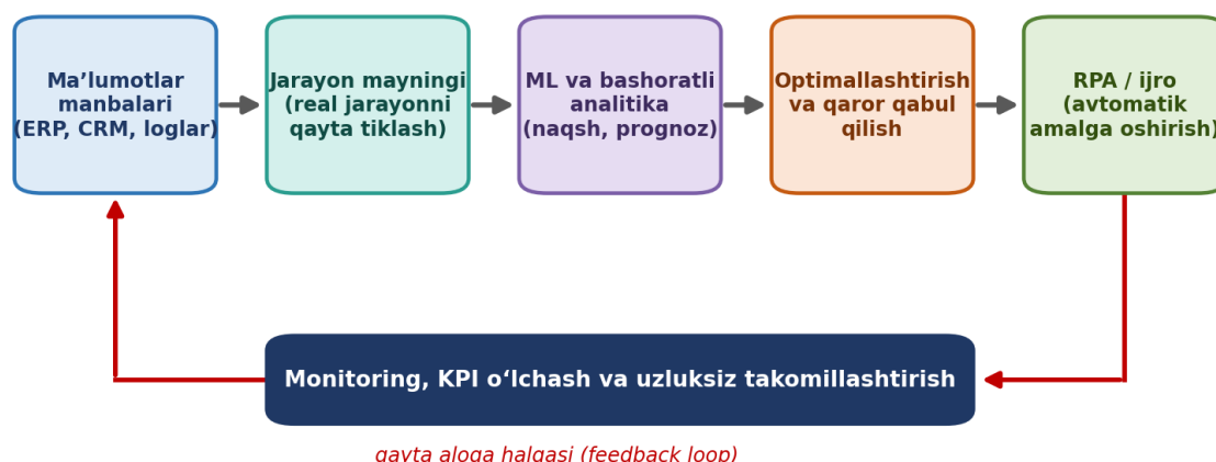
5-rasm. Intellectual jarayon avtomatlashtiruv quvurining (pipeline) arxitekturas
